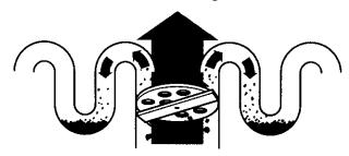
8. Soil in the ULTRA WASH Soil Removal System is disposed down the drain with the wash water.
